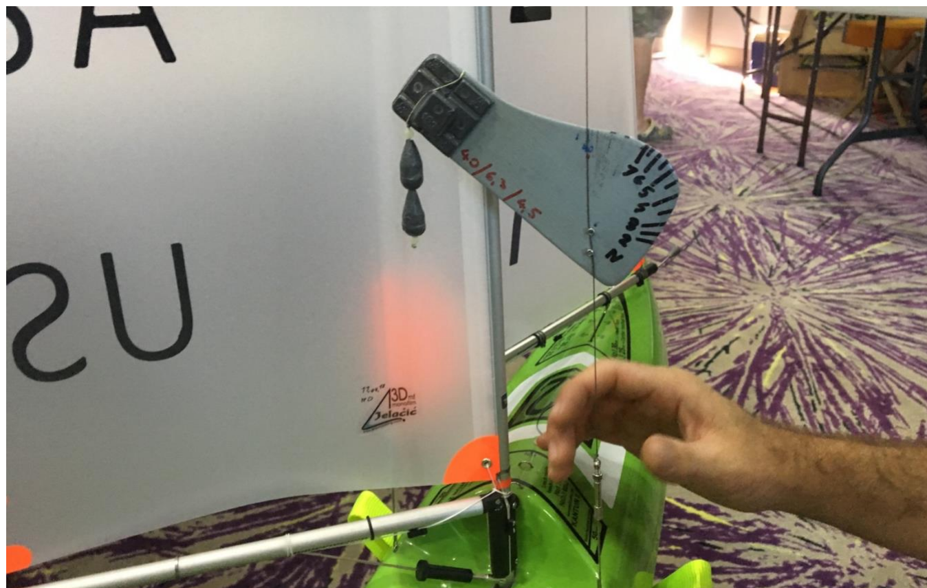
2017 IOM Nats at Garland, TX; and my new K2 is getting a rig setup by designer Zvonko Jelacic. That's his shroud tension meter in neutrons, and he uses lead weights and gravity to measure the tension.
